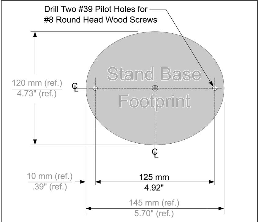
Figure 13. Stand Base Hole Pattern (Not to Scale)
