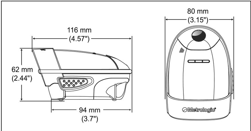
Figure 2. Scanner Dimensions
