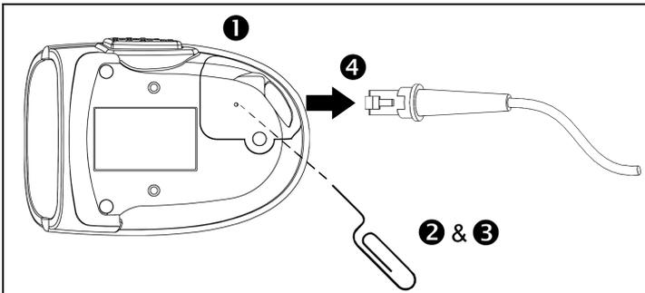
Figure 7. Releasing the PowerLink Cable
