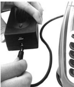
☛ Then connect the other cable to the power supply unit and connect the twin pronged electrical plug to an electrical point
