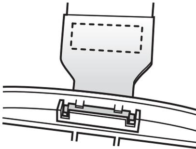
**Figure 1-16** Pin and Handstrap in Mounting Area
