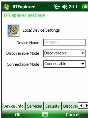
**Figure 5-28** BTE Explorer Settings - Device Info Tab
