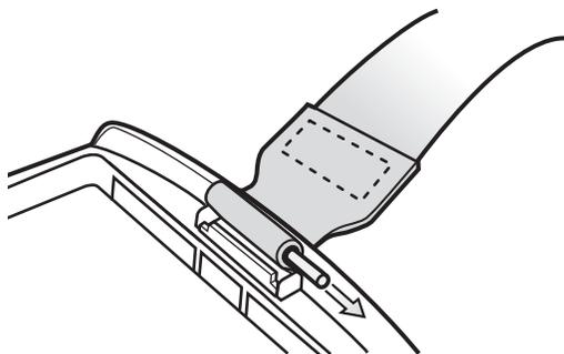
**Figure 1-14** *Pin Removal*
