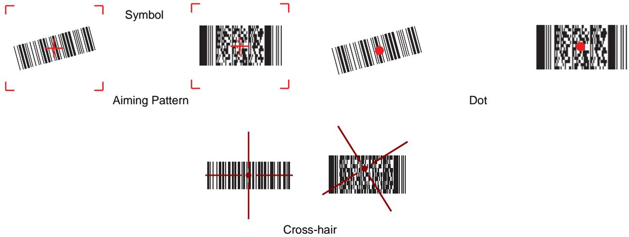
**Figure 2-26** Imager Aiming Pattern: Bar Code Centered
