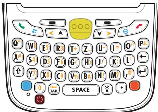
**Figure 2-19** QWERTZ Keypad Configuration
