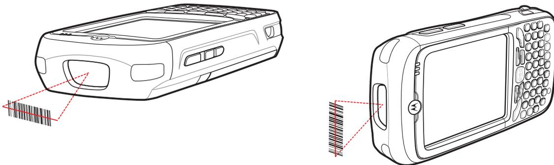
**Figure 2-23** *Linear Scanning*
