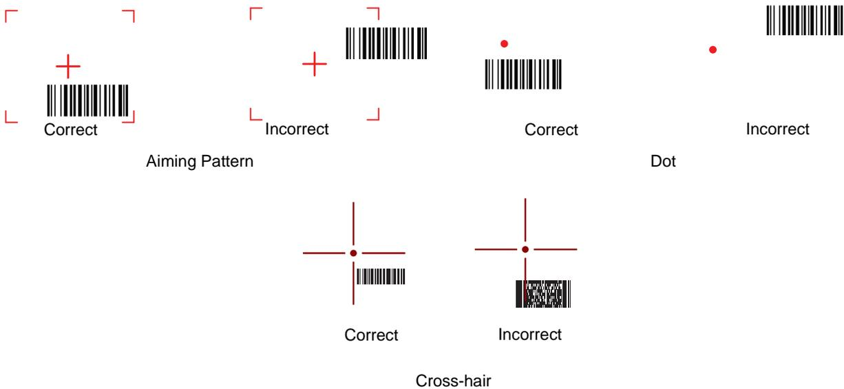
**Figure 2-27** Imager Aiming Pattern: Bar Code Not Centered
