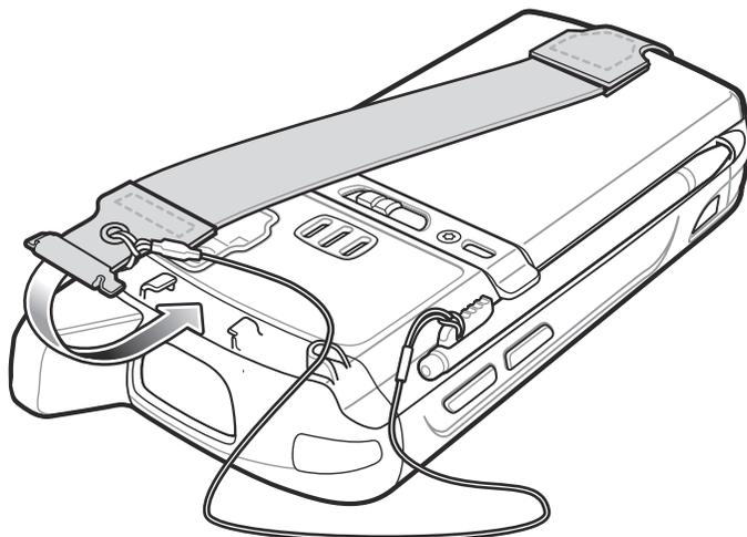
**Figure 1-17** Slide Handstrap and Tether Over Handstrap Mount
