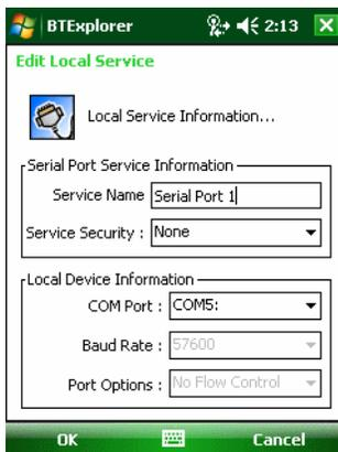
**Figure 5-38** BTE Explorer Settings - Serial Port Services
