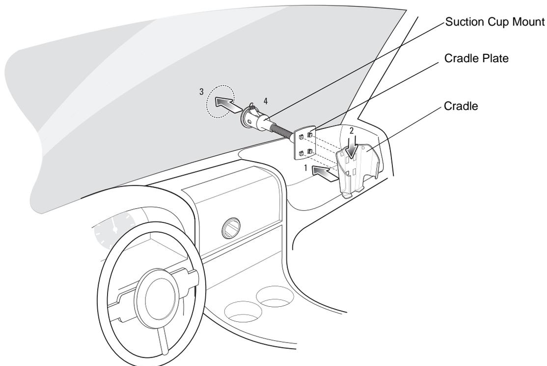
**Figure 6-13** *Windshield Installation*
