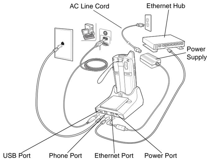
**Figure 6-3** Connection Setup
