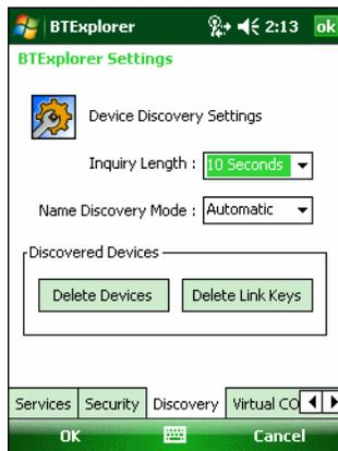
**Figure 5-42** BTE Explorer Settings - Discovery Tab**Table 5-15** Discovery Tab Data
