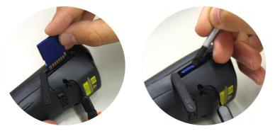
To remove the SD card, just push it toward the inside, aided by the back of the stylus, until it clicks; a spring system will return it out.
