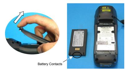
4. Install the new battery pack, first insert the bottom (contacts) side, then the upper (lock) side as indicated in the following figure:
