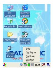
By selecting the *Info* item from this drop-down menu you can access information about the Scanner and the Software; the *Configure* item opens the configuration applet (Data Capture Configuration Window), while *Capture* accesses the data capture applet (Data Capture Window), which enables code reading. The last menu item (*Wedge*) enables Wedge Emulation.
