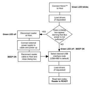
Successive start-ups will automatically recognize the previously loaded drivers. If external power is used, verify that external power is already supplied.
