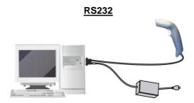
With the RS232 cable, this accessory device is intended to be supplied by a UL Listed or CSA Certified Direct Plug-in Power Unit marked "Class 2", rated 5 V, minimum 180 mA.
