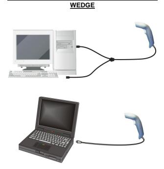
With the Wedge or PC Notebook cables, this accessory device is intended to be connected to either a UL or CSA Certified Listed Computer which supplies power directly to the reader or a UL Listed or CSA Certified Direct Plug-in Power Unit marked "Class 2", rated 5 V, minimum 180 mA.
