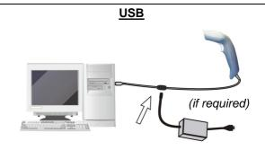
With the USB cable, this accessory device is intended to be supplied by a UL Listed or CSA Certified Power Unit marked "Class 2", or an LPS power source which supplies power directly to the reader.
